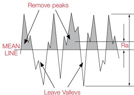
improved surface finish allows contact loading to be distributed over more surface area reducing contact stress and extending pitting fatigue life.
